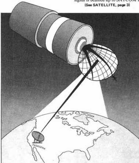
SATELLITE SYNDICATION — The above illustration pictures how the Work's Media Services Department will transmit the World Tomorrow telecast through the Westar IV satellite to selected Canadian and U.S. stations. The Work now uses the SATCOM I satellite. [Artwork by Ron Grove]
