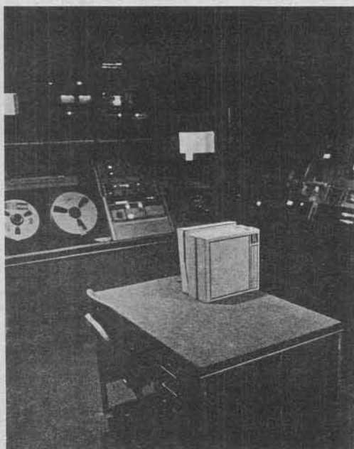
COMPUTERIZED EDITING — The CMX300, a completely computerized electronic editing system, allows continuous 24-hour editing of the telecast. It can pinpoint any individual frame, of which 30 pass per second. [Photo by Bruce Voyce]
